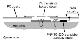
TR2 acts as a temperature sensor, so the best place to track temperature variations is to bolt TR2 to the heatsink, very close to the flange of the PA transistor TR1.
