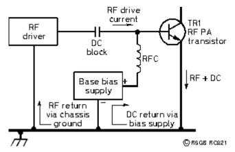
In this circuit, RF drive turns on TR1 and makes it draw both base and collector current. The RF return path is via TR1 emitter and chassis ground - but the DC return path is through the bias supply. This means that the bias supply must be capable of delivering the full DC base current at maximum RF drive.
